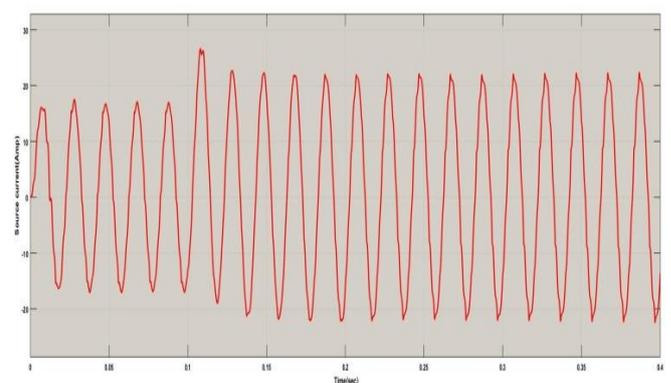
**Fig -6:** Source current waveform with hybrid filter compensation
