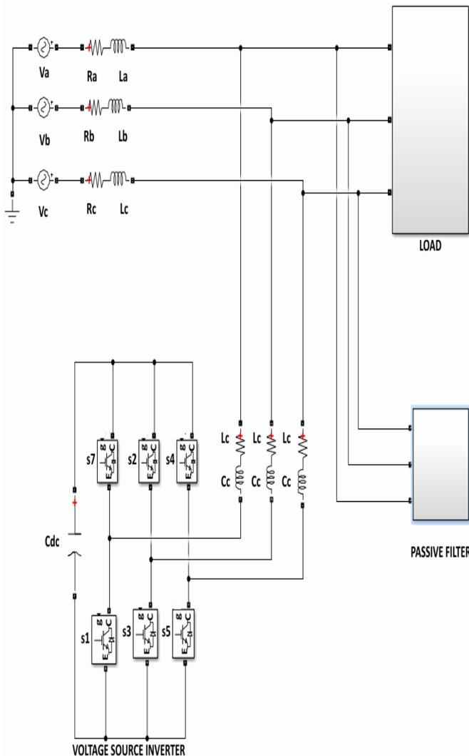
Fig -2: Hybrid Filter with Combination of Shunt Active and Shunt Passive Filter
