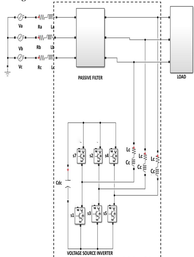
Fig1; Hybrid Filter with Combination of Series Passive and Shunt Active Filter
