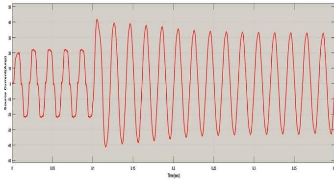
**Fig -7:** Source current waveform without filter compensation
