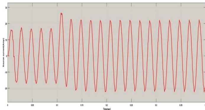
**Fig 8:** Source current waveform with compensation
