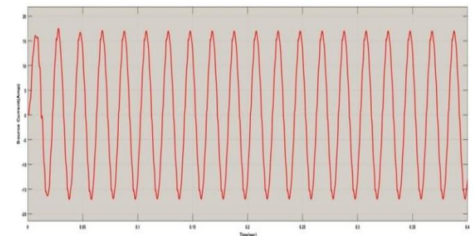
**Fig -5:** Source current waveform with passive filter only
