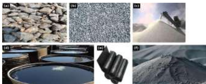
Fig -1: Materials used in the study — (a) coarse aggregate; (b) fine aggregate; (c) filler material (M-sand); (d) cutback; (e) cement; (f) waste plastic
