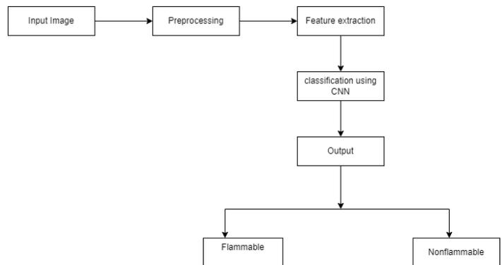
Recent advancements in image processing have allowed vision-based systems to detect fire using Convolutional Neural Networks during surveillance. Two custom CNN models have been implemented for a cost-effective fire detection CNN architecture for surveillance videos. To balance the efficiency and accuracy, the model is fine-tuned considering the nature of the target problem and fire data. We are going to use three different datasets for training our models.
