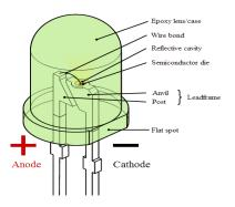
A **light-emitting diode** (**LED**) is a semiconductor light source. LEDs are used as indicator lamps in many devices and are increasingly used for other lighting.
