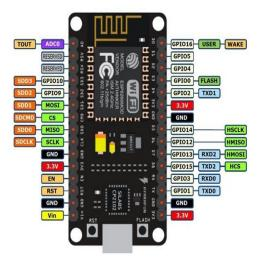
NodeMCU is an open-source Lua based firmware and development board specially targeted for IoT based Applications. It includes firmware that runs on the ESP8266 Wi-Fi SoC from Espressif Systems, and hardware which is based on the ESP-12 module.
