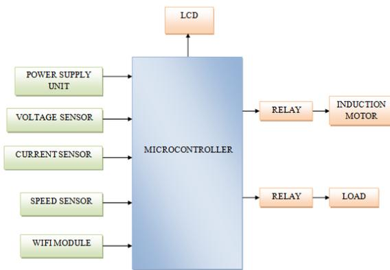
Fig.No: 3.1 Block Diagram Industrial Device Control Using Wi-Fi Module
