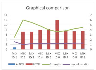
From above results we can clearly say that compressive strength is affected by various factors like modulus ratio, alkali liquids, water content, fly ash and GGBS content and percentage of rising agent.
