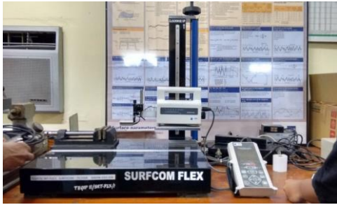
Figure 3: Surfcom FLEX 50-Aused for Measuring surface roughness.
