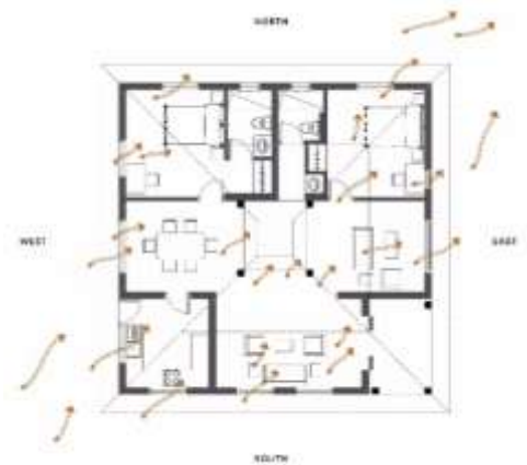
Fig- 2: Orientation of windows and openings, aligned to face internal courtyards
