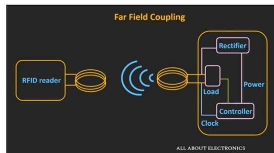
matching across the coil if the load is matching exactly the in-backscatter signal will be more. If the load is not matched exactly the intensity of the backscatter signal is less if we change the condition of the load according to the data that is stored in a database across the RFID chip the data can send back to the RFID reader initial signal sent by the reader is strong.
