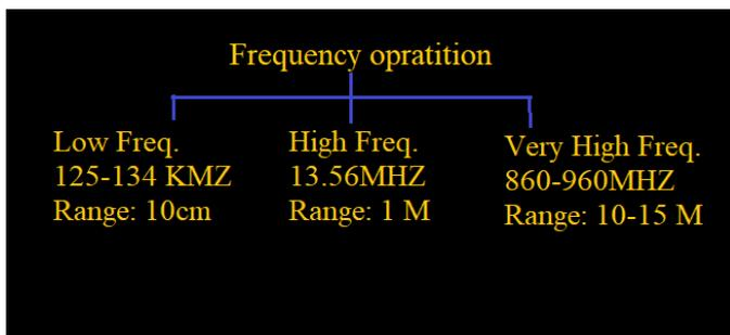
The majority of the company uses a Very High-Frequency level in RFID chip. As low-frequency signal travel from a short distance the range of the RFID chip is up to 10 cm. high-frequency signal travel greater than low frequency the range of the RFID chip is up to 1M. very high-frequency ravel longer than both frequency 10-15 M.
