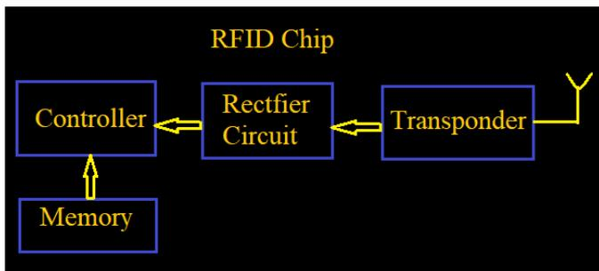
from the reader using this rectifier circuit energy from radio wave across the capacitor. This energy is used as a supply for the controller as well as the memory of the RFID chip.
