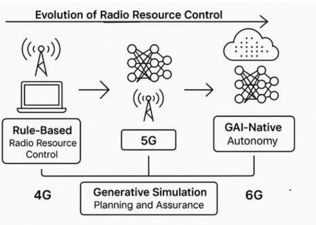
shows the conceptual evolution from rule-based radio resource control to GAI-native autonomy across  $4G \rightarrow 5G \rightarrow 6G$ , highlighting the role of generative simulation for planning and assurance.
