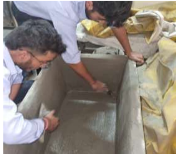
Figure 5. Construction of Prototype Tank with 12.5% Tyre Rubber Crumb
