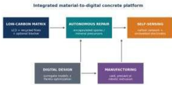
Fig. 1. Proposed integrated architecture linking material functions, digital design, and manufacturing.
