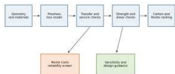
Fig. 2. Integrated analysis sequence used to connect structural response, embodied carbon, and uncertainty.
