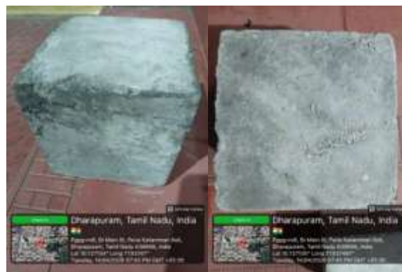
Fig. 12: Sulphate Attack Test Specimens after Exposure
