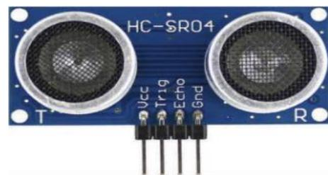
Fig 2. Ultrasonic sensor
