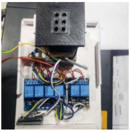
Hardware Integration: Pins connected to solenoids controlled through MOSFET drivers
