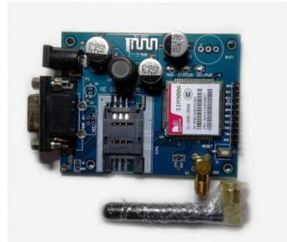
Fig -8: GSM SIM900
