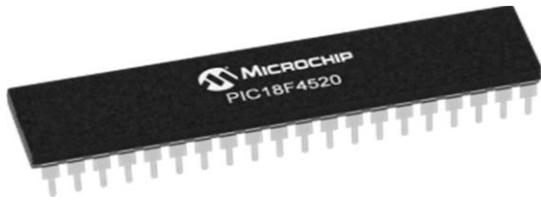
Fig -2: PIC 18f4520 Microcontroller
