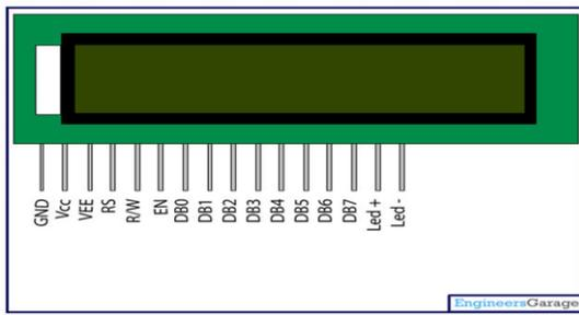
Fig -3: LCD Display
