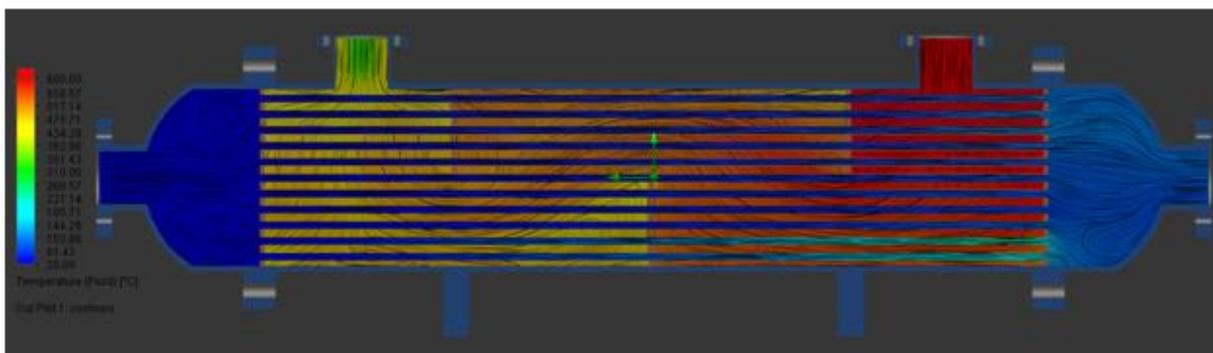
*Figure 6. Temperature distribution in a heat exchanger*
