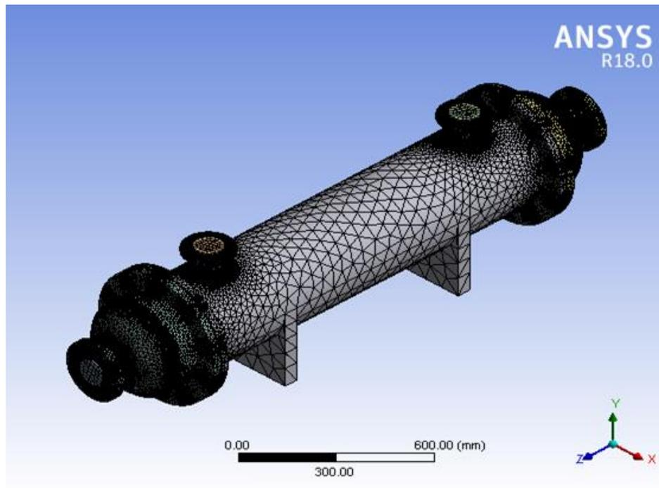
**Figure 4. Meshing view of a heat exchanger**
