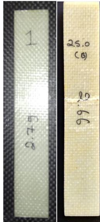
FIGURE 7. Test specimen after Compression Testing
