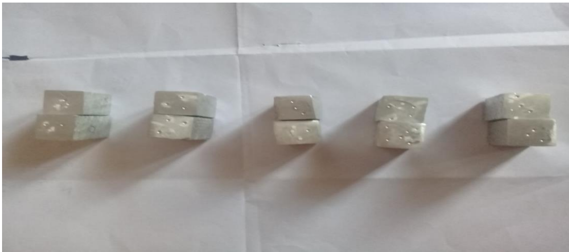
Fig 5.3 Hardness Test Sample Specimen
