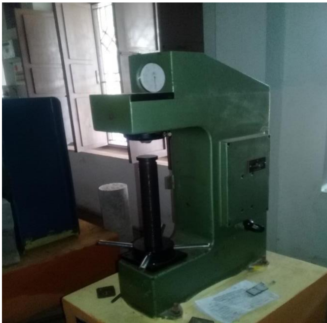
Fig 6.3 : Rockwell hardness testing machine
