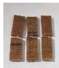
Tensile tested specimen of 30% ATH
