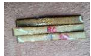
Fig.5.12 Flexural test specimen with 10% ATH
