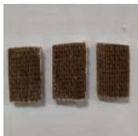
Fig.5.21 hardness tested specimen with 0% ATH Fig.5.22 hardness test specimen with 10% ATH
