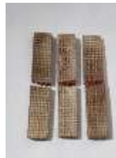
Fig.5.17 impact tested specimen with 0% ATH Fig.5.18 impact test specimen with 10% ATH
