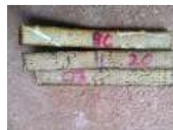
Fig.5.11 Flexural tested specimen with 0% ATH
