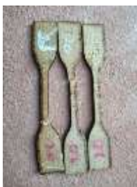
Tensile tested specimen Of 20% ATH
