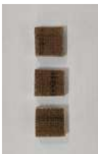
Fig.5.21 hardness tested specimen with 0% ATH Fig.5.22 hardness test specimen with 10% ATH
