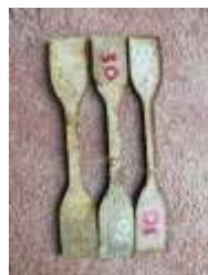
Tensile tested specimen of 30% ATH
