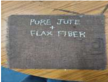
Fig 5 preparation of specimen without ATH
