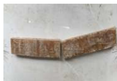
Fig : 14 impact test (After testing)
