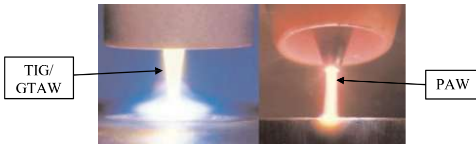
Fig. 1.1: A comparison of the TIG/GTAW (left) and Plasma (right) welding arcs [4]
