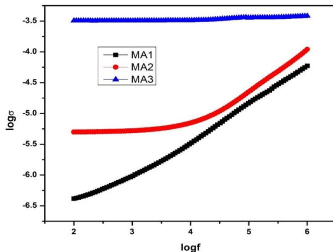
**Figure 5:**  $\log f$  vs.  $\log \sigma$  of  $Mg(ClO_4)_2$  salt added PVC/ZnO nanocomposite polymer electrolytes
