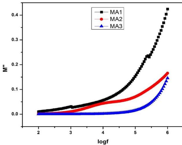
**Figure 4:** Frequency vs. imaginary part of electric modulus of  $Mg(ClO_4)_2$  salt added PVC/ZnO nanocomposite polymer electrolytes
