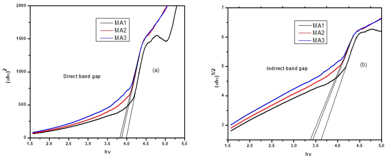
**Figure 2 (a&b):** Direct and indirect bandgap plots of  $Mg(ClO_4)_2$  salt added PVC/ZnO nanocomposite polymer electrolytes
