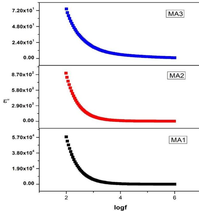
**Figure 7:** log f vs.  $\epsilon''$  of  $\text{Mg}(\text{ClO}_4)_2$  salt added PVC/ZnO nanocomposite polymer electrolytes
