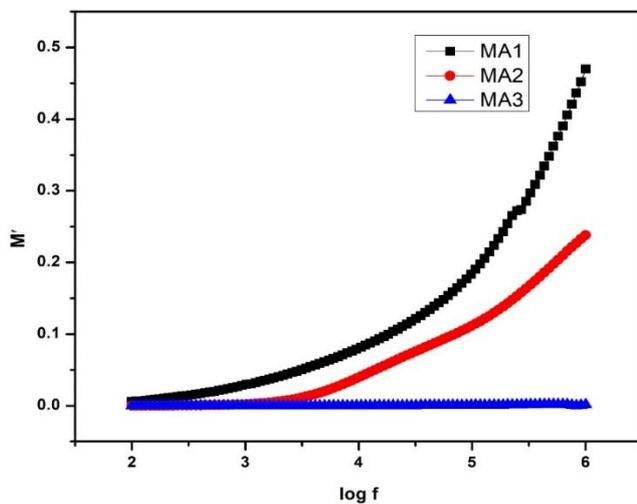
**Figure 3:** Frequency vs. real part of electric modulus of  $Mg(ClO_4)_2$  salt added PVC/ZnO nanocomposite polymer electrolytes
