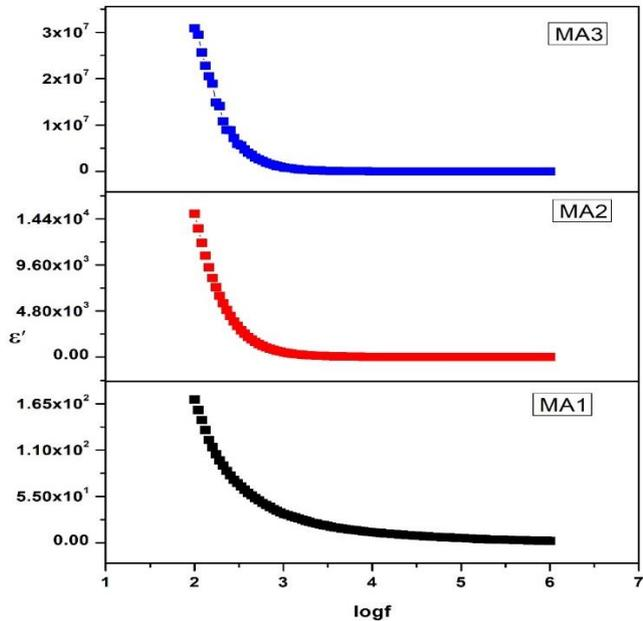
**Figure 6:** log f vs.  $\epsilon'$  of  $\text{Mg}(\text{ClO}_4)_2$  salt added PVC/ZnO nanocomposite polymer electrolytes
