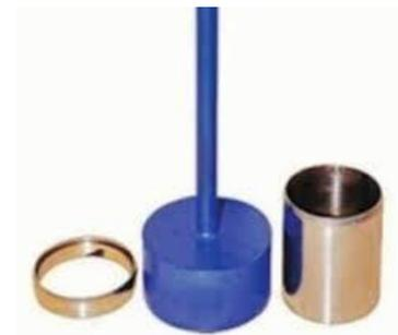
Fig- 1 steel rammaer
