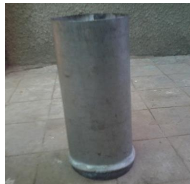
Figure 15: Deformed Cylinder after Testing
