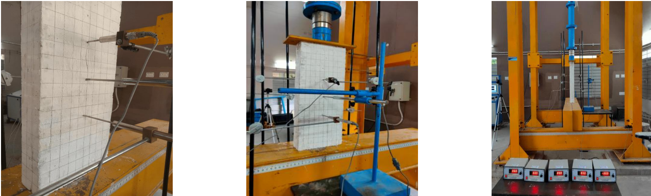
Fig :5 Testing arrangement for wall panel
