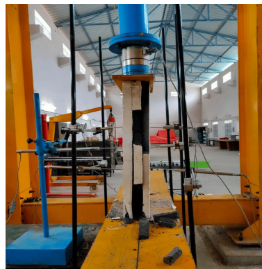
Fig :8 Failure pattern of wall panel
