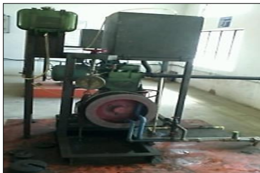
Fig5:4-stroke single cylinder engine diesel engine setup
