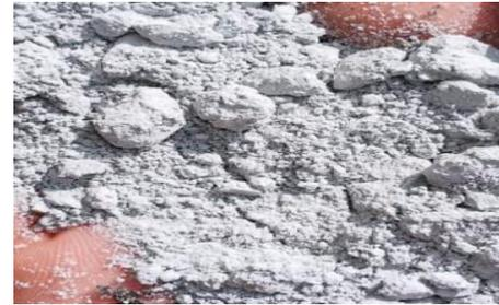
Fig 1: Sample of granite waste powder
