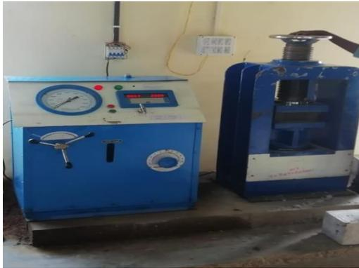
**Fig 3: Compression testing machine of concrete paver block**
