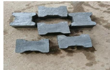
Fig 2: Sample of concrete paver block after casted
