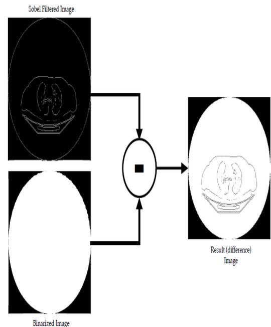
**Figure 3.3: Creation of the mask that will be employed for the removal of the gantry artifact**
