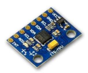
MPU6050 sensor module is complete 6-axis Motion Tracking Device. It combines 3-axis Gyroscope, 3-axis Accelerometer and Digital Motion Processor all in small package. Also, it has additional feature of on-chip Temperature sensor. It has I2C bus interface to communicate with the microcontrollers.
