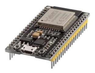
Typically, the ESP32 is embedded on device-specific printed circuit boards or offered as part of development kits that include a variety of <u>GPIO</u> pins and connectors, with configurations varying by model and manufacturer. The ESP32 was designed by <u>Espressif Systems</u> and is manufactured by <u>TSMC</u> using their 40 nm process. [2] It is a successor to the <u>ESP8266</u> microcontroller.
