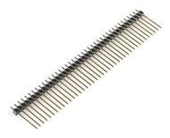
Pin headers are stiff metallic connectors that are soldered to a circuit board and stick up to receive a connection from a female socket.
