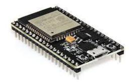
The ESP32 is a series of low-cost, low-power system-on-a-chip microcontrollers with integrated Wi-Fi and dual-mode Bluetooth. Espressif Systems, a Chinese business with its headquarters in Shanghai, designed and developed the ESP32, which is produced by TSMC.
