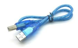
USB stands for Universal Serial Bus. It is used as a data cable for programming as well as for supplying power.
