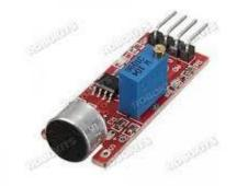
A sound sensor can detect the sound intensity of the environment. The main component of the module is a simple microphone, which is based on the LM386 amplifier and an electret microphone.
