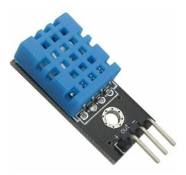
The DHT11 is a commonly used temperature and humidity sensor. The sensor comes with a dedicated NTC to measure temperature and an 8-bit microcontroller to output the values of temperature and humidity as serial data. The sensor is also factory calibrated, making it easy to interface with other microcontrollers.
