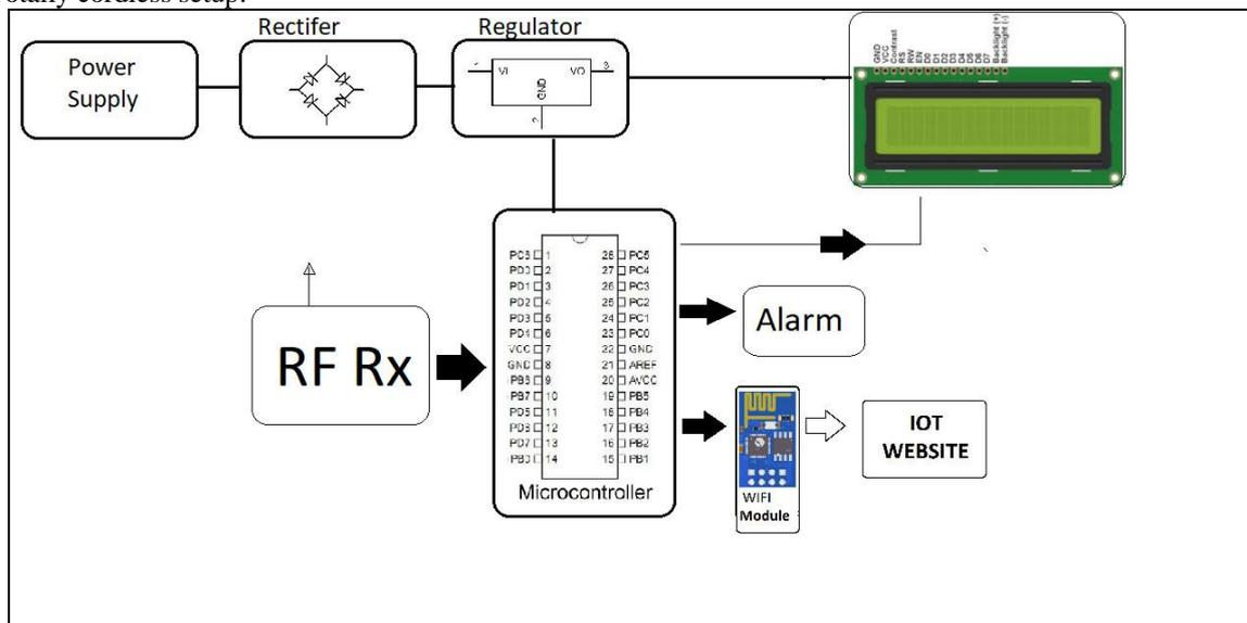
Figure 1. Transmitter block diagram of coal mine safety monitoring system
