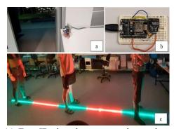
**Figure 3.** (a) Two IR obstacle sensor nodes at the entrance to track people in and out; (b) ToF sensor node to track front desk violation; (c) addressable LED strip (ws2812b) based visual markers for the queue (green: allowable, red: no-go area).
