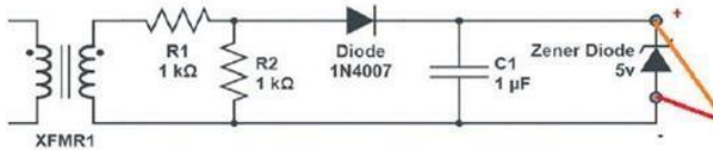
Figure 4. Voltage Measurement Circuit
