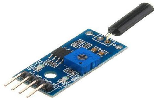
Fig.3: Vibration Sensor
