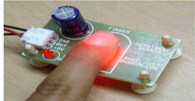
Fig.7: Heart Rate monitoring Sensor
