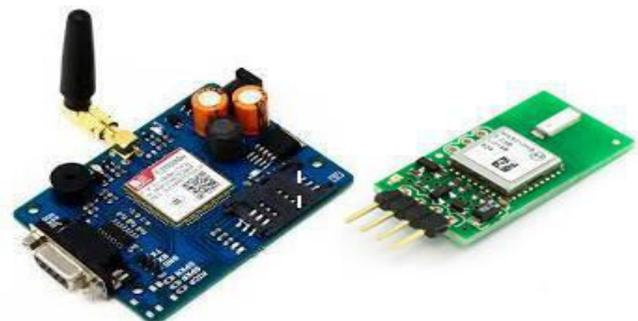
Fig.4: GSM and GPS Module
