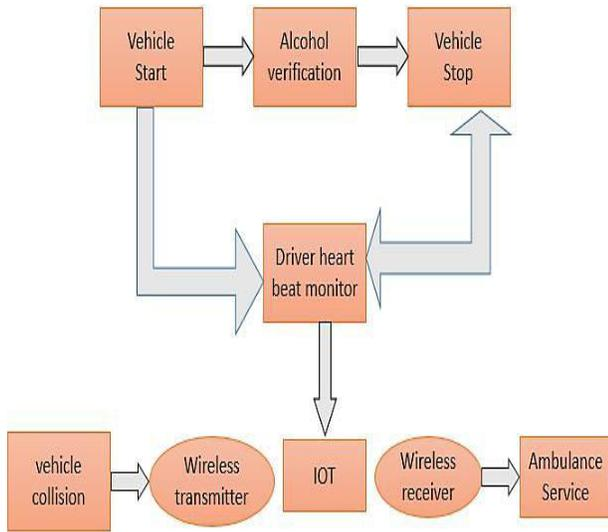
Fig. 5: System Architecture
