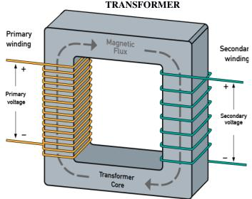
• Transformers convert AC electricity from one voltage to another with little loss of power. Transformers work only with AC and this is one of the reasons why mains electricity is AC.
