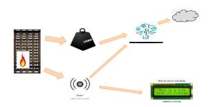
or fire. Logic low on output indicates absence of flame or fire.
