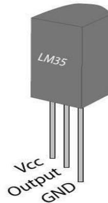
LM35 is a precision IC temperature sensor with its output proportional to the temperature (in °C). The sensor circuitry is sealed and therefore it is not subjected to oxidation and other processes. With LM35, temperature can be measured more accurately than with a thermistor. It also possess low self-heating and does not cause more than °C temperature rise in still air.
