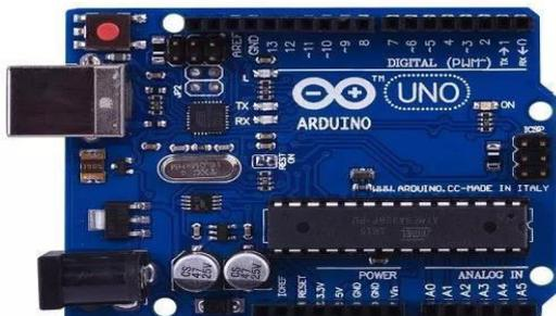
The Arduino Uno has a number of facilities for communicating with a computer, another Arduino, or other
