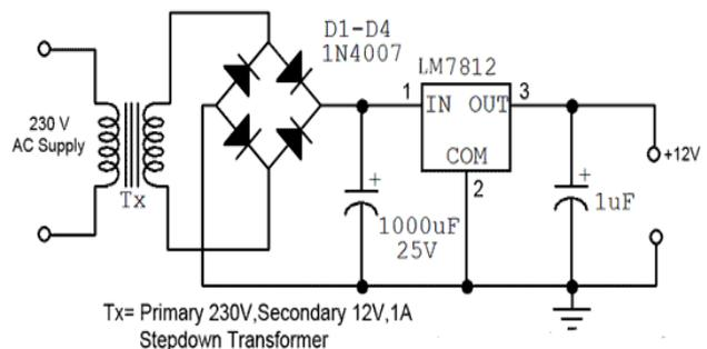
Power supply is a reference to a source of electrical power. A device or system that supplies electrical or other types of energy to an output load or group of loads is called a power supply unit or PSU. The term is most commonly applied to electrical energy supplies, less often to mechanical ones, and rarely to others.
