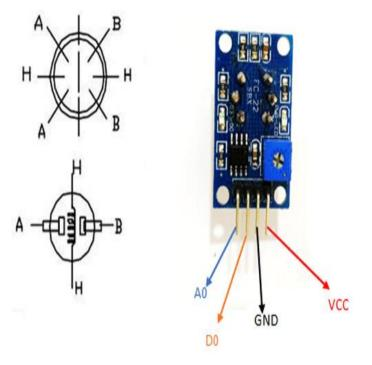
MQ4 is a gas sensing module, which is used to measure methane gas in the atmosphere. It contains Gas sensing layer, which is made up of SnO2. SnO2 is sensitive to gases like LPG, CH4, H2, CO, Alcohol, and smoke. As the decaying food emits methane gas (CH4), the MQ4 sensor can be used to measure this gas to monitor food quality. You can also check this \_project where we used a similar gas sensor to monitor air quality by measuring PPM.
