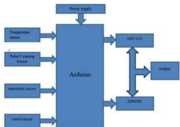
Fig.1. Block Diagram Of Health Monitoring System
