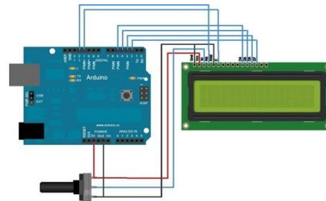
Figure.7 Interfacing of Arduino Uno and LCD Display
