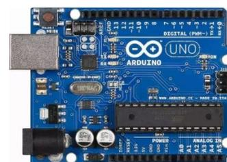
Figure.4 Arduino Uno Microcontroller
