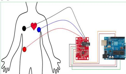
Figure.6 Interfacing of AD8232 and Arduino Uno[5]
