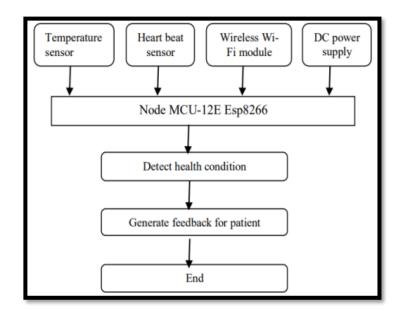
Fig.6.1.System architecture of healthcare monitoring using IoT
