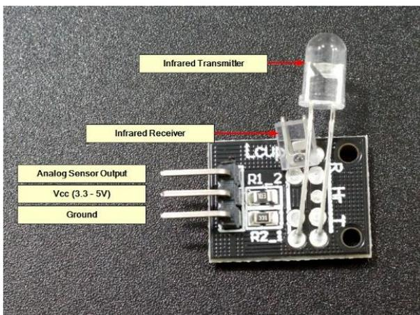
Fig-4: Heart Rate Sensor Module
