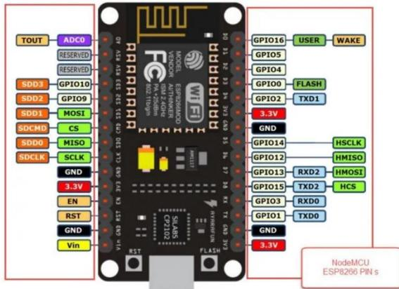
Fig -3: Microcontroller NODE MCU
