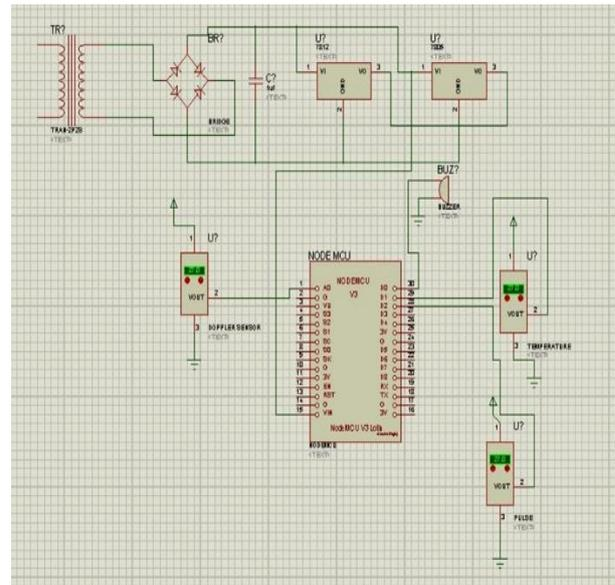
Fig-9: Simulation of the working system
