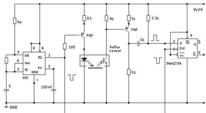
Fig-10: Working of Pulse Sensor with Buffer storage
