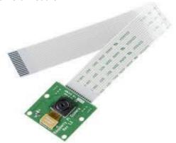
Camera module is the pi camera interfacing to the raspberry pi module. It is used to capture images and send them to the pi module. The LED flashes to handle the light condition that is supplied by the environment and these are called as ambient light conditions.
