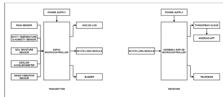
Fig.1 Block Diagram of Landslide Detection System
