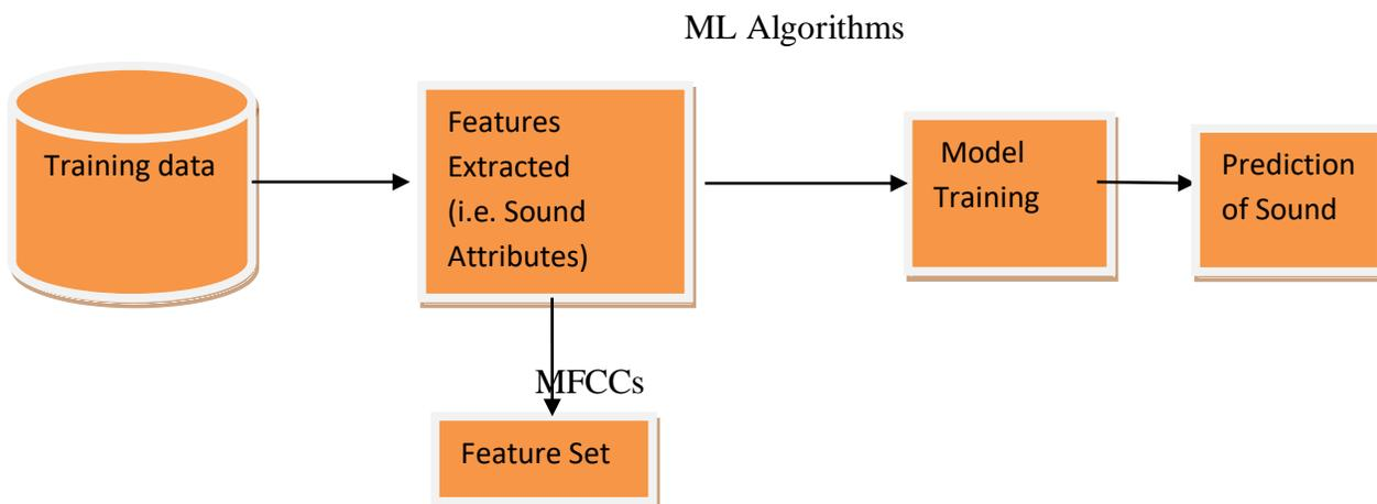
Figure 1: Approach for machine sound identification using machine learning
