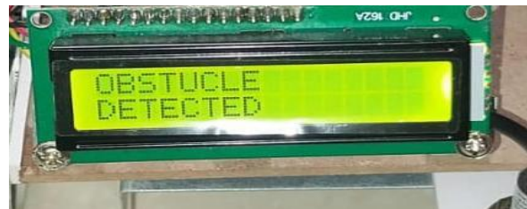
Fig.11.: Display Picture of Obstacle Detected
