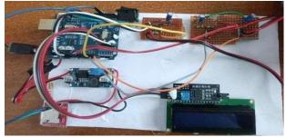
Fig.2 : Model Picture of IOT based power theft detection and smart energy metering
