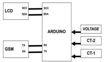
**Fig. 1:** Block diagram of IOT based power theft detection and smart energy metering
