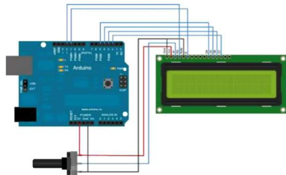
Fig. 3. Wiring schematic for LCD-Arduino interfacing
