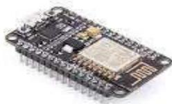
Fig. 2.ESP8266-12E board
