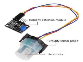
A turbidity sensor is an analytical sensor that measures turbidity. They are highly useful and effective instruments to identify the clarity and particle content in a solution, like water. Turbidity sensors are used to reduce waste, improve yields, and analyze water quality in a wide range of industries.
