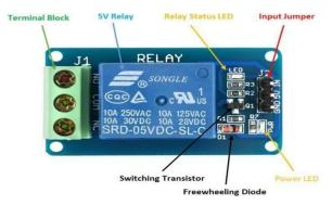
A relay channel in a smart irrigation system controls a water pump. It serves as a switch that can be remotely operated to start or stop the pump, allowing for efficient and automated irrigation. This technology enables precise control over water distribution in agricultural fields, conserving resources and optimizing crop growth.
