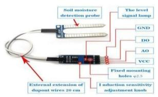
Soil moisture sensor using a measuring moisture level and get moisture level like a Dry or wet, normal.Dry: (520 430], Wet:
