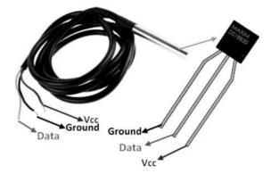
As this is a 1-wire digital temperature sensor, it needs only the data pin and GND pin to interface with the Arduino or microcontroller. The temperature sensing of the sensor ranges from - $55^{\circ}$ C to +125°C with an accuracy of  $\pm 5^{\circ}$ C. It is the best temperature sensor to measure the temperature value at multiple points and requires only one data/digital pin of the Arduino or microcontroller unit to transfer the data.
