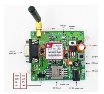
**Data Communication:** The Arduino uno connects to a GSM module, typically via UART communication. The GSM module has a SIM card for cellular data access.
